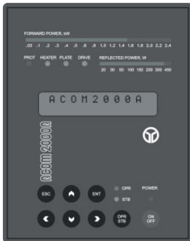
Fig.3-1 Remote Control Unit (RCU)
